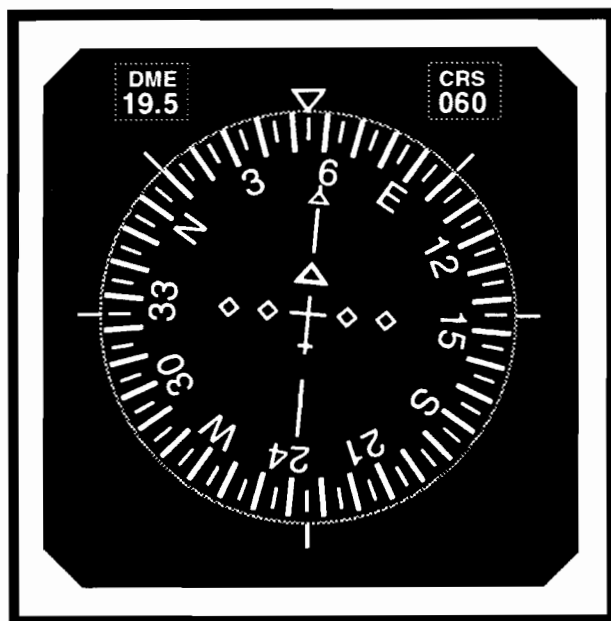
FIGURE 113.—Aircraft Course and DME Indicator.
