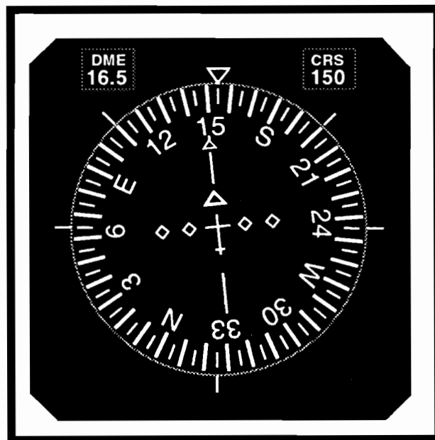
FIGURE 114.—Aircraft Course and DME Indicator.
